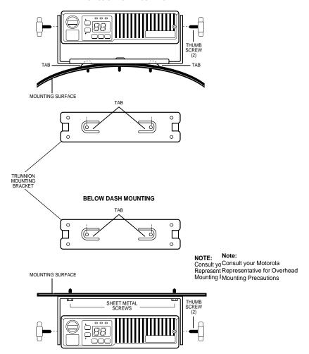
Figure 4. Trunnion Mount for Radio
