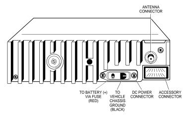
Figure 3. Connections to Rear Radio Panel
