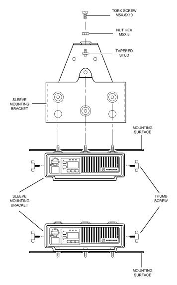
Figure 5. Sleeve Mount for Radio
