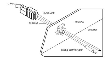
Figure 1. DC Power Cable Routing into Engine Compartment
