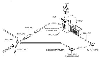
Figure 2. DC Power Cable Assembly
